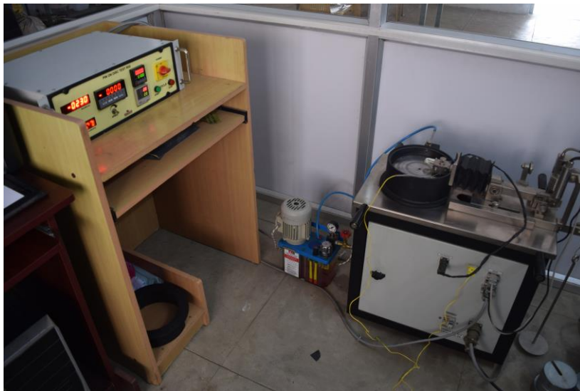
Pin on Disc Friction and Wear Test Rig
