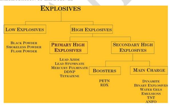
**1. Propellants** or **low explosives** are combustible materials, containing within themselves all oxygen needful for their combustion, which burn but do not explode, and function by producing gas which produces an explosion. Under normal conditions, low explosives
