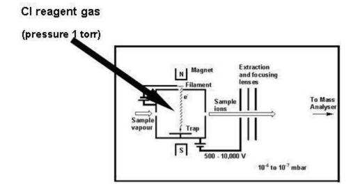
Figure 2. Schematic diagram of CI interface
