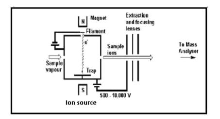
Figure 1. Schematic diagram of EIMS
