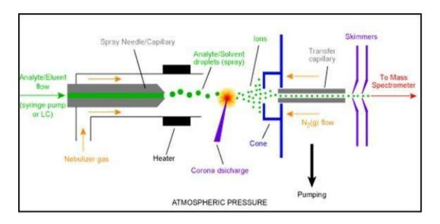
In general, proton transfer occurs in the positive mode to yield [M+H]+ ions. In the negative ion mode, either electron transfer or proton loss occurs to yield M- . or [M-H]- ions, respectively. The moderating influence of the solvent clusters on the reagent ions, and of the
