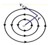
Schematic representation of a vortex flow.
