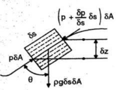
The body force is  $\rho Fs \, \delta A \, \delta s$ . On the upstream face the pressure force is  $p \, \delta A$  in the (+s) direction and on the downstream face it is  $\left(p + \frac{\partial p}{\partial s} \, \delta s\right) \, \delta A$  acting in the (-s) direction. The total force along the path  $\delta s$  with tangential unit vector is given by
