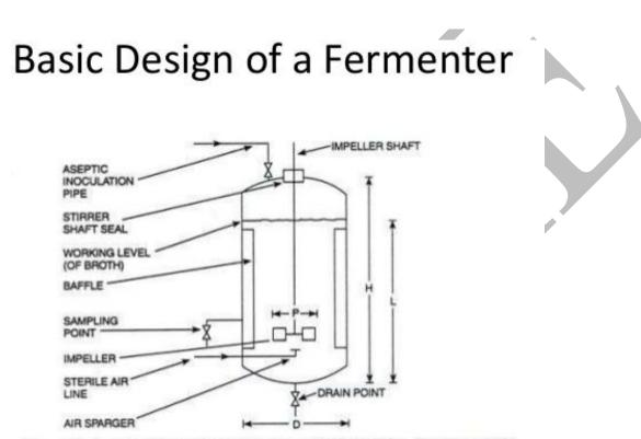
Diagram of a fermenter with one multi-bladed impeller. H, fermenter height; L, liquid height; D, tank diameter; P, impeller diameter.
