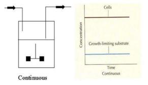
(1) A steady-state condition of the total number of cells and the total volume in the bioreactor is maintained.
