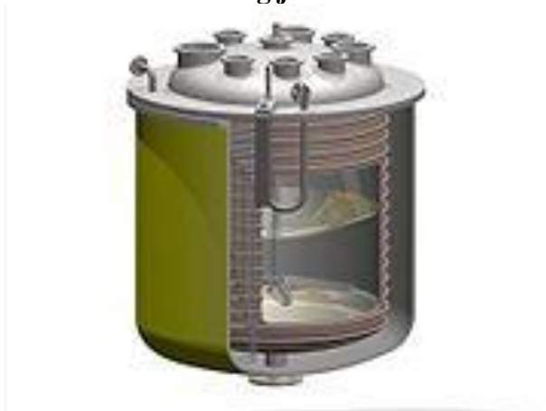
Batch reactor with constant flux (Coflux) jacket
