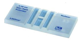
Neubauer's chamber is a thick glass plate with the size of a glass slide (30x70x4mm). The counting region consists of two square shaped ruled areas. There are depressions or the moats on either side or in between the areas on which the squares are marked thus giving an "H" shape.
