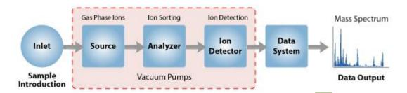
Figure: Components of a Mass Spectrometer
