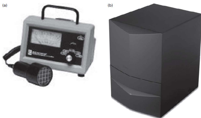
Fig. 14.4 (a) Geiger-Mueller bench monitor; (b) liquid scintillation counter
