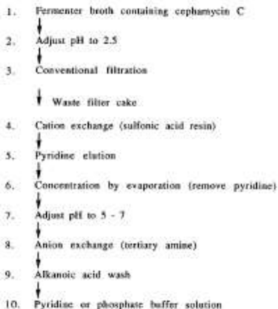
FIG. 10.3. Purification of cephamycin C: sequential ion exchange process (Omstead et al. , 1985).
