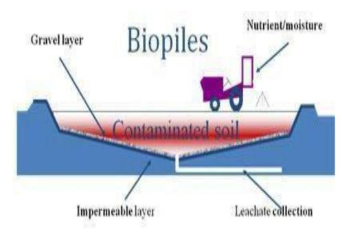
The treatment area will generally be covered or contained with an impermeable liner to minimize the risk of contaminants leaching into uncontaminated soil. The drainage itself may be treated in a bioreactor before recycling. Vendors have developed proprietary nutrient and additive formulations and methods for incorporating the formulation into the soil to stimulate biodegradation. The formulations are usually modified for site-specific conditions.
