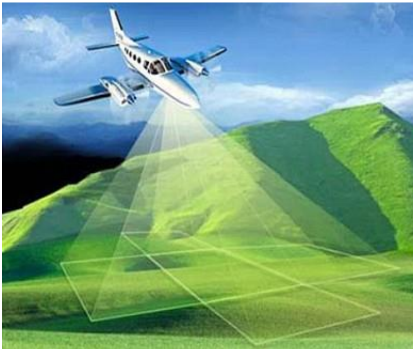
Figure 1.8 Configuration of Pictometry imaging
