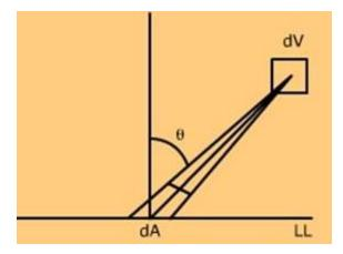
Let us first discuss the average no. of molecules crossing the surface xx from above. Consider an element of volume dV at distance r from an element area dA in the plane xx' and the direction makes an angle  $\theta$  with normal to the plane. Let n be the number density so that the
