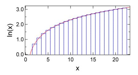
The sum of the area under the blue rectangles shown below up to N is ln N!. As you can see the rectangles begin to closely approximate the red curve as m gets larger. The area under the curve is given the integral of ln x.
