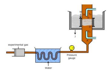
A **porous plug** consists of silk fiber or cotton wool packed in a space between two perforated brass discs (DD) and has a number of fine holes such that heat cannot flow smoothly through it and this process is considered to be adiabatic. Thus, porous plug maintains a constant pressure difference on the opposite sides of the plug.
