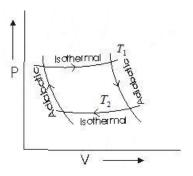
(i) In step b $\rightarrow$ c isothermal expansion of gas taken place and thermodynamic variables of gas changes from (P<sub>1</sub>, V<sub>1</sub>,T<sub>1</sub>) to (P<sub>2</sub>,V<sub>2</sub>,T<sub>1</sub>)
