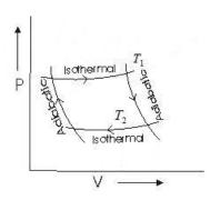
(i) In step b $\rightarrow$ c isothermal expansion of gas taken place and thermodynamic variables of gas changes from (P<sub>1</sub>, V<sub>1</sub>,T<sub>1</sub>) to (P<sub>2</sub>,V<sub>2</sub>,T<sub>1</sub>)
