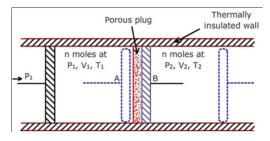
The dotted lines in the figure indicate the final position of the piston.
