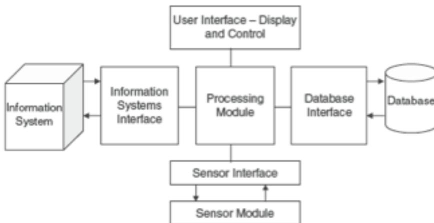
Fig 1: Architecture of a virtual instrument
