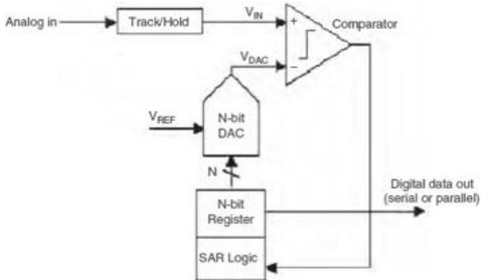
**Fig 11: Simplified N-bit SAR ADC architecture**
