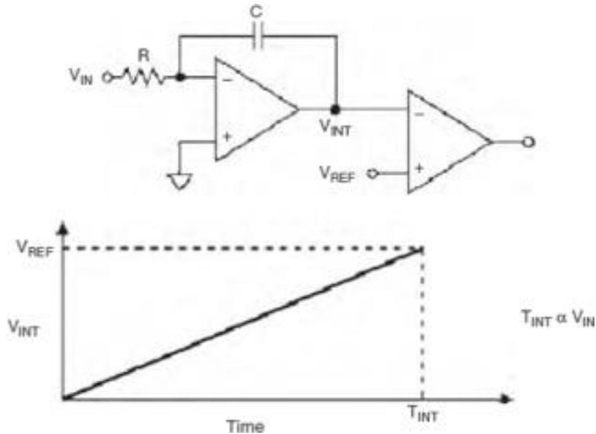
**Fig 8:(a) Single-slope ADC circuit (b) Response of single slope ADC**
