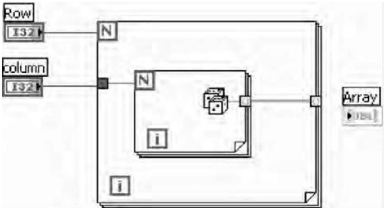
Fig14: For loop for creating 2 D array
