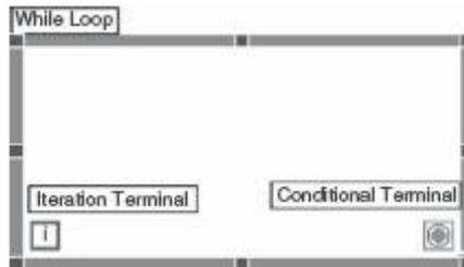
Fig 4: While loop terminals
