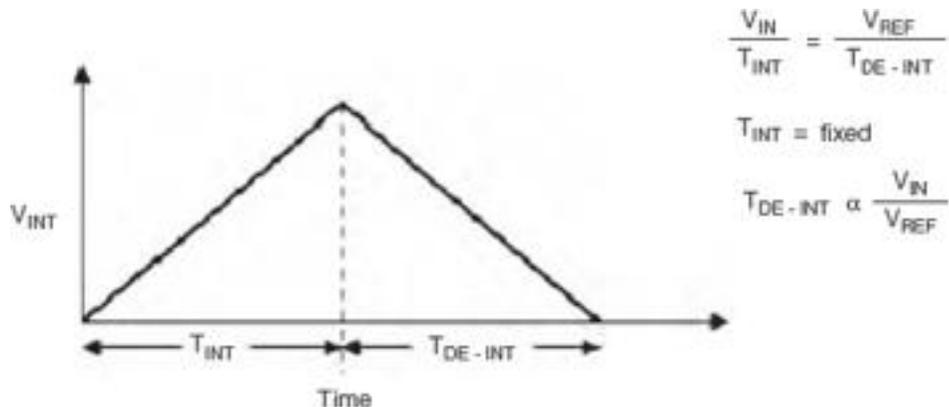
**Fig 9: Dual slope integration**
