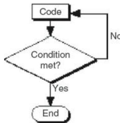
Fig 5: Flowchart of while loop
