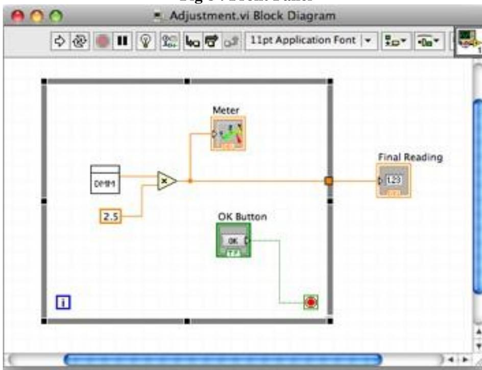
**Fig 9: Block diagram of multimeter**
