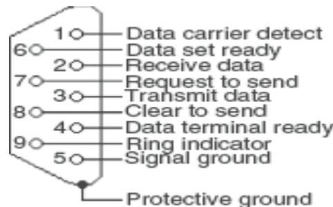
**Fig 3: Pin diagram**
