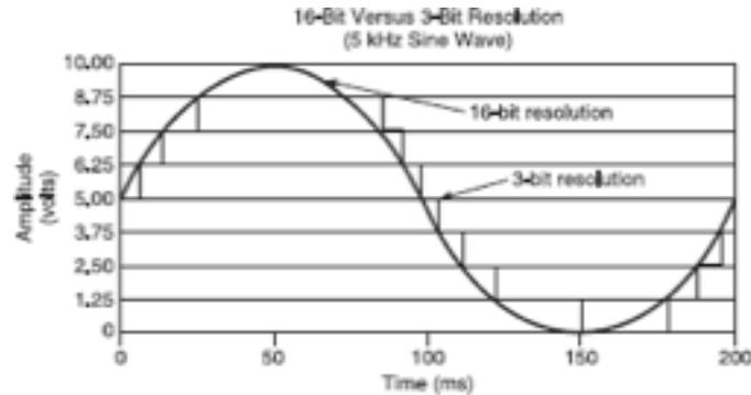
**Fig : 3 bit and 16 bit resolution**
