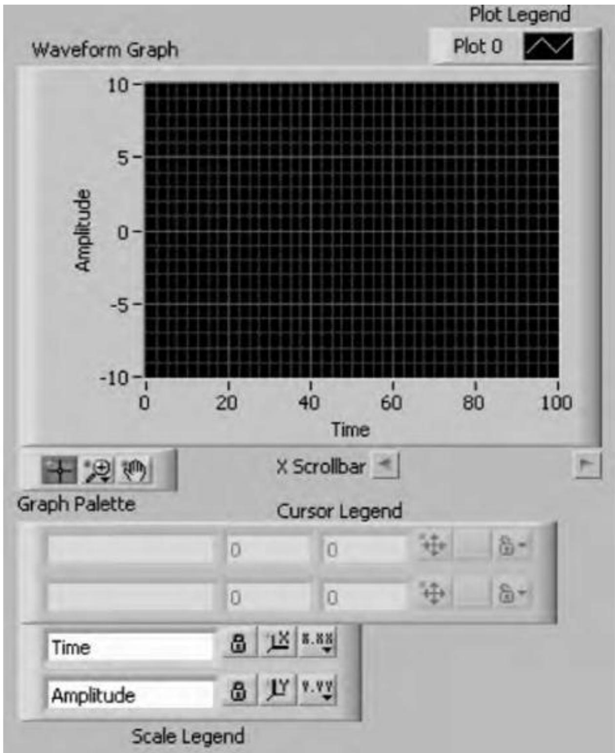
Fig 22: waveform graph
