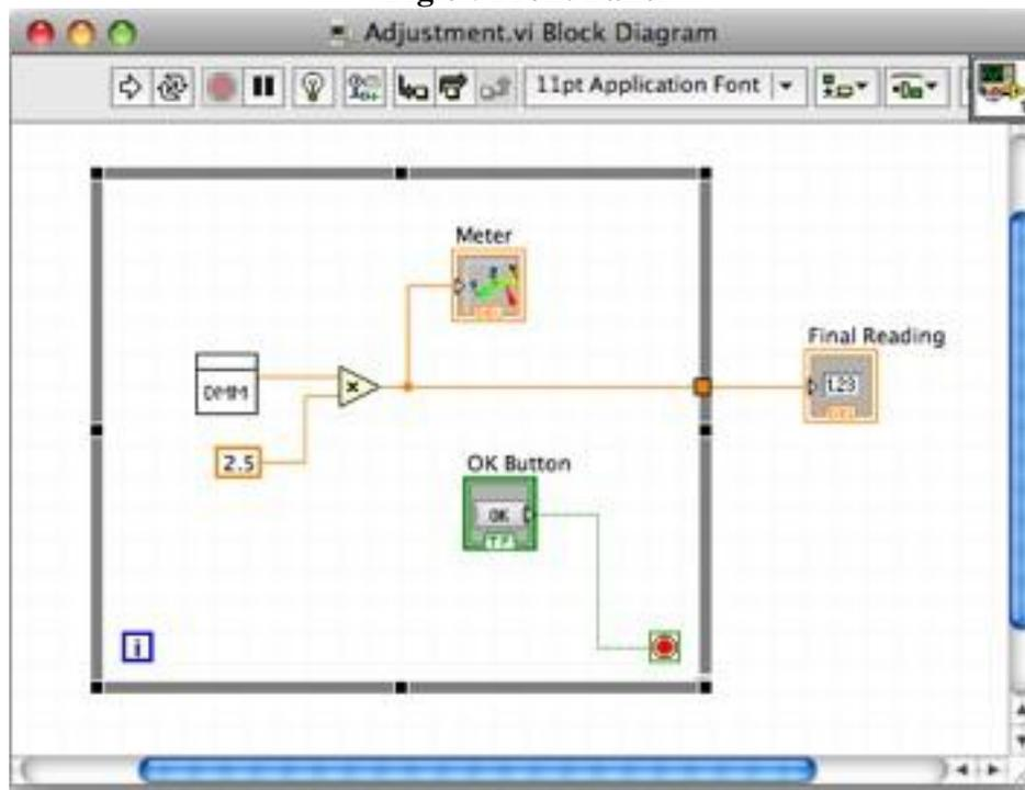
**Fig 9: Block diagram of multimeter**
