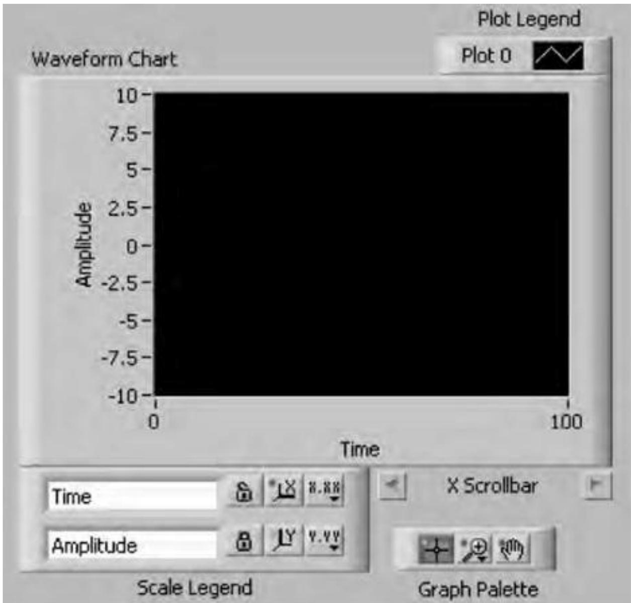
**Fig24: Waveform chart and its component**
