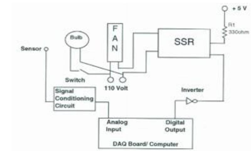
**Fig 4: ON-OFF Temperature Control
