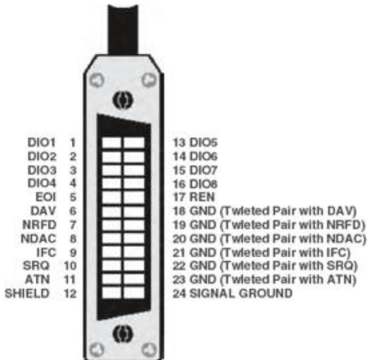
**Fig :6 Bus structure of GPIB**
