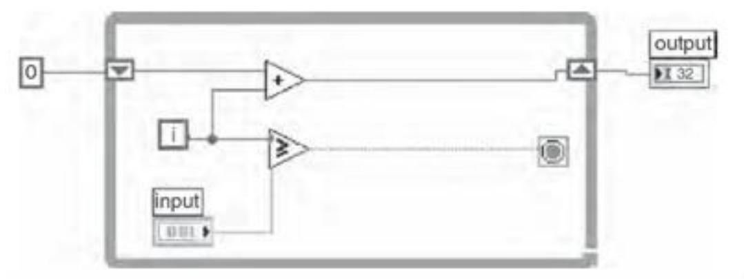
Fig 9: Block diagram of while loop for the above example
