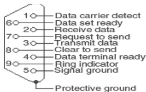
**Fig 3: Pin diagram**
