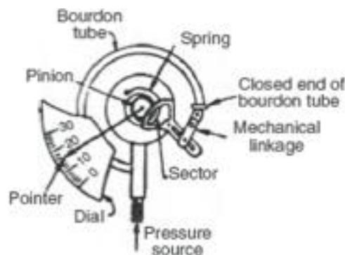
**Fig 3: Bourdon tube pressure gauge**
