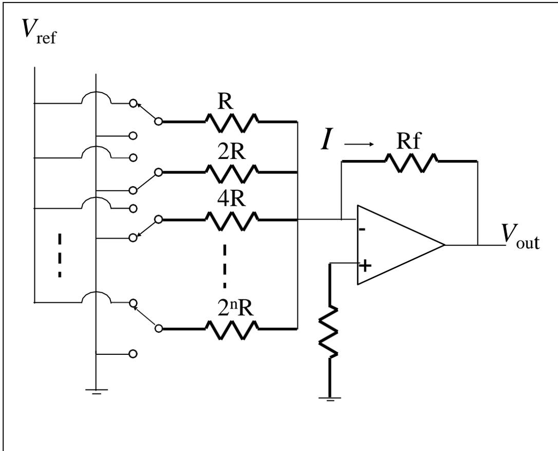
Fig 13: Binary Weighted Resistor
