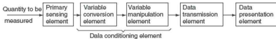
**Fig 2: Functional elements of an instrumentation system**
