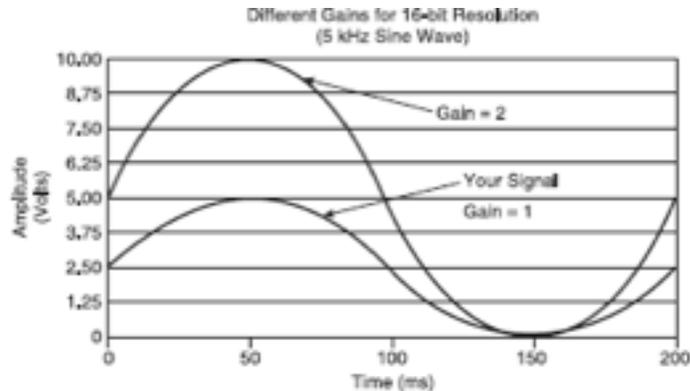
**Fig : Effects of applying amplification in resolution using the following formula**
