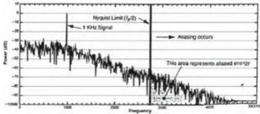
**Fig 5: Power spectrum of a 1 kHz sine wave with low pass-filtered noise added**
