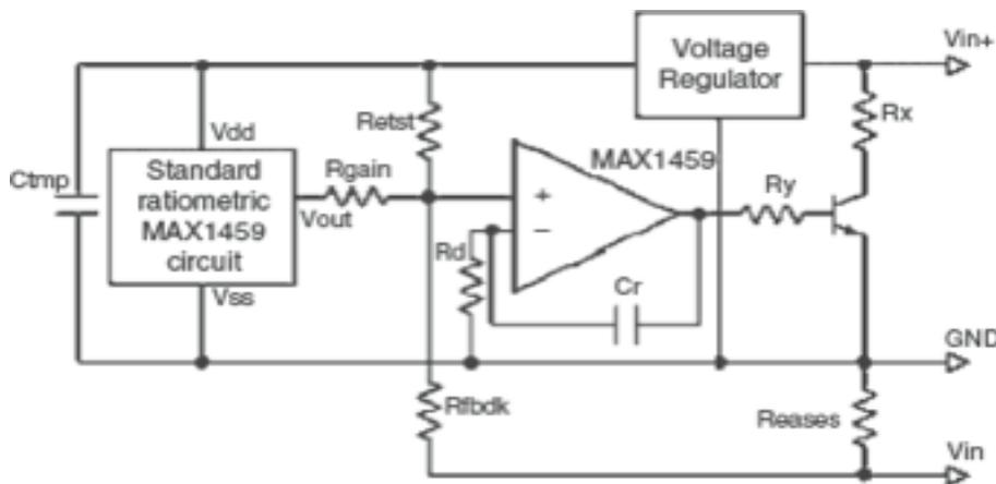
**Fig2: 4-20 mA transmitter**
