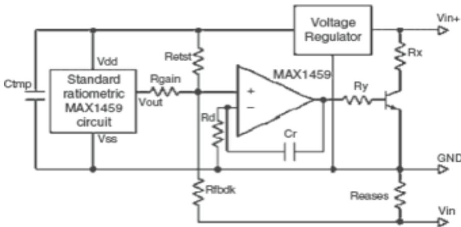
**Fig2: 4-20 mA transmitter**
