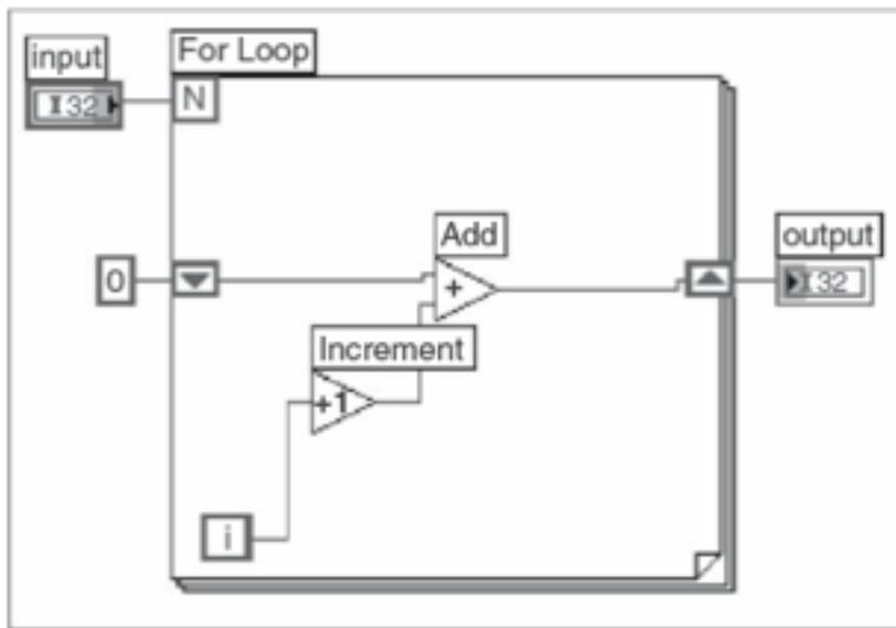
Fig 7: Block diagram of for loop example
