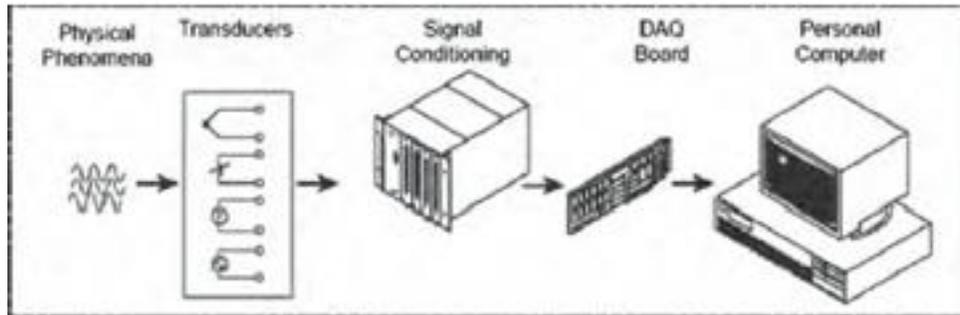
**Fig 1: A general PC-based DAQ system with signal conditioning**
