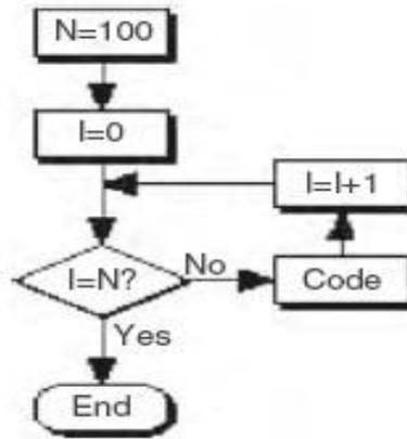
Fig 2: Flow chart of For loop
