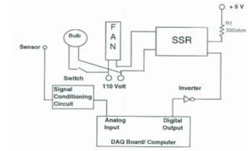
**Fig 4: ON-OFF Temperature Control
