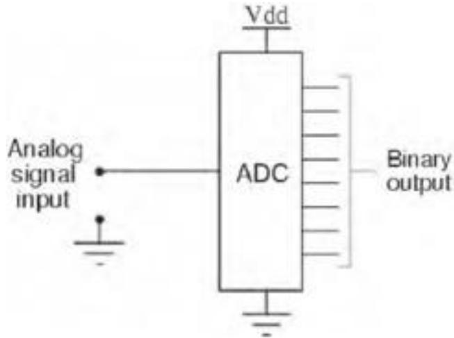
**Fig 7: Analog-to-digital converter**
