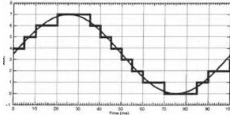
**Fig 6: A sine wave and its representation by a 3-bit ADC sampling every 5 ms**
