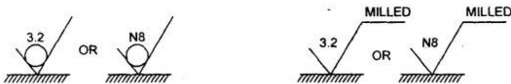
Fig. 1.9 Indication of surface roughness in micrometers or roughness grade symbols
