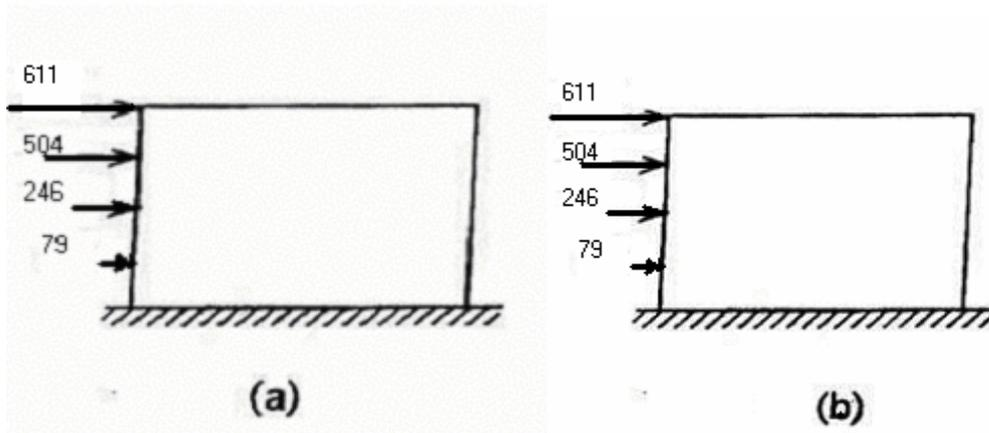
**Figure 1.2 -- Design seismic force on the building for (a) X-direction, and (b) Y-direction.**
