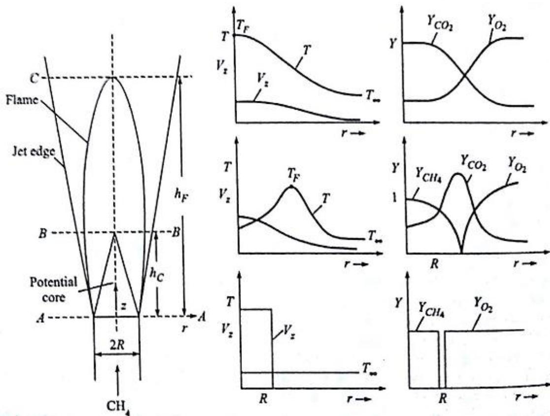
The flame structures of laminar gaseous jet diffusion flame.
