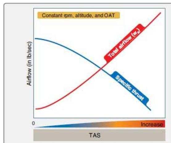
*Fig. 6 Effect of airspeed on net thrust.*
