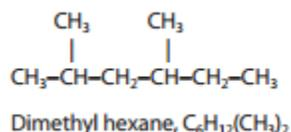
Current aviation fuels contain an average of 60% paraffins, depending on the source of the crude oil and the distillation process. In general, paraffins tend to have a higher hydrogen/carbon ratio, lower density, lower freeze point, and high gravimetric calorific value than other types of hydrocarbon fuels.
