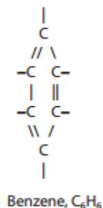
More complex molecules of the aromatic group are obtained either by replacing one or more of the hydrogen atoms with hydrocarbon groups or by "condensing" one or more rings [8]. Another example is:
