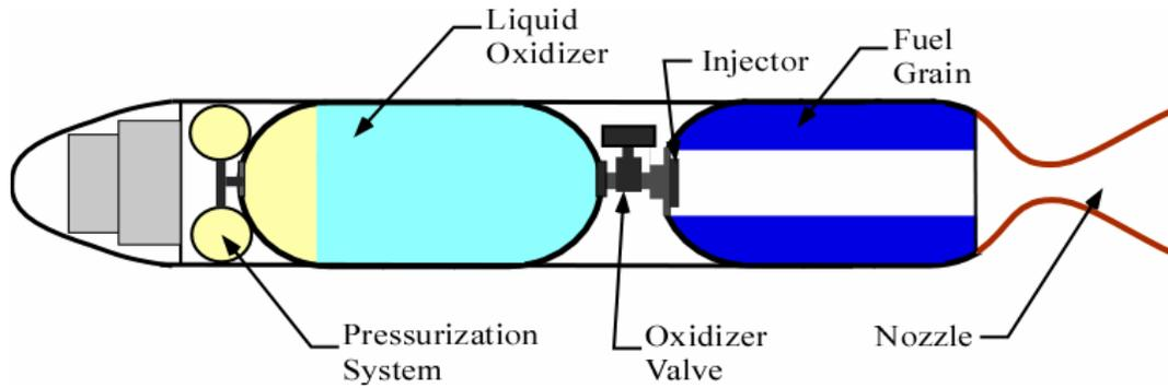
Fuel and oxidizer are physically separated One of the two is in solid phase.
