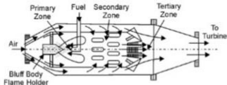
Combustion Chamber with Upstream Injection with Bluff-body Flame Holder.
