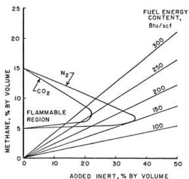
Flammable fuel mixtures of CH<sub>4</sub>-N<sub>2</sub> and CH<sub>4</sub>-CO<sub>2</sub> at one atm showing various energy levels.
