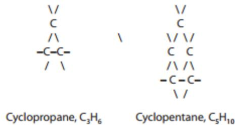
Naphthenes are major constituents of jet fuel, i.e., about 25–35%. They closely resemble paraffins in their chemical stability, high gravimetric heat of combustion, and low soot-forming tendencies.
