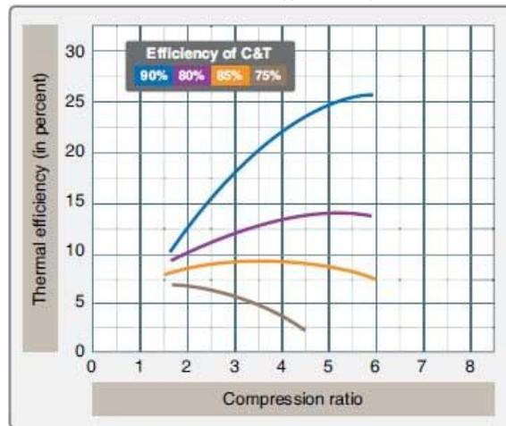
Fig. 2. *Turbine and compressor efficiency vs. thermal efficiency.*
