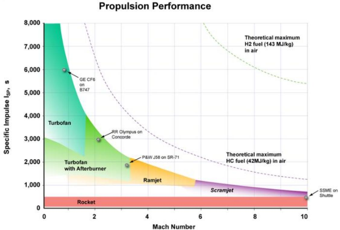
The performance of a [launch system](#) is complex and depends greatly on its weight. Normally craft are designed to maximise range (R), orbital radius (R) or payload mass fraction ( $\dot{r}$ ) for a given engine and fuel. This results in tradeoffs between the efficiency of the engine (takeoff fuel weight) and the complexity of the engine (takeoff dry weight), which can be expressed by the following:
