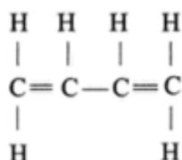
The polybutadiene chain structure is  $-(\text{CH}_2=\text{CH}-\text{CH}=\text{CH}_2)_n-$ . Here  $n$  is the number of butadiene groups. The polybutadiene chain could be attached to poly-acrylo-nitrile group and acrylic acid groups given by:
