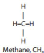
The remaining normal paraffins are built up from methane as straight chains, e.g.
