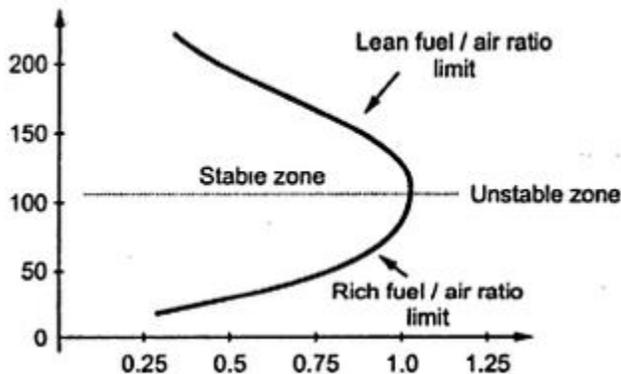
For any combustion the flame will be stable depending on fuel/air ratio quality. Flame may blow out at lean fuel/air or at rich fuel/air mixture. This is taken as limit of stability, in which flame will hold. Normally instability will occur before the lean or rich fuel/air ratio limit is reached. Instability of flame indicates poor combustion, sets up aerodynamic vibrations which ultimately reduces
