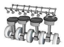
A typical 2-valve engine has just 1/3 combustion chamber head area covered by the valves, but a 4-valve head increases that to more than 50%, hence smoother and quicker breathing. 4-valve designs also benefit a clean and effective combustion, because the Spark Plug can be placed in the middle.
