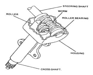
The cam and lever steering uses one or two lever studs fitted in taper roller bearing. When the worm in the form of helical groove rotates the stub axle and it also rotates along with it. This imports a turning motion to the drop arm shaft.
