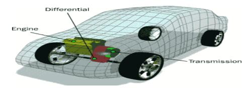
Front-wheel drive (or FWD for short) is a common form of internal combustion engine / transmission layout used in modern passenger cars, where the engine drives the front wheels. Using the front wheels for delivery of power as well as steering allows the driving force to act in the same direction as the wheel is pointing.
