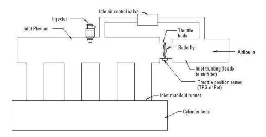
Single-point injection uses a single injector at the throttle body (the same location as was used by carburetors).
