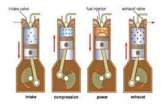
The diesel engine has the highest thermal efficiency of any standard internal or external combustion engine due to its very high compression ratio. Low-speed diesel engines (as used in ships and other applications where overall engine weight is relatively unimportant) can have a thermal efficiency that exceeds 50%.
