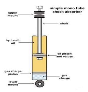
By these hydraulic actions and reactions, the shock absorbers permit a soft ride over small valves and provide firm control over spring action for cushioning large bumps. The double – acting units operate efficiently in both directions. Spring rebound can be almost as violent as the original action that compressed the shock absorber.
