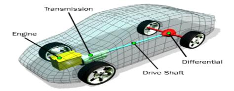
Rear-wheel drive (or RWD for short) was a common internal combustion engine / transmission layout used in automobiles throughout the 20th century. RWD typically places the engine in the front of the vehicle, but the mid engine and rear engine layouts are also used.
