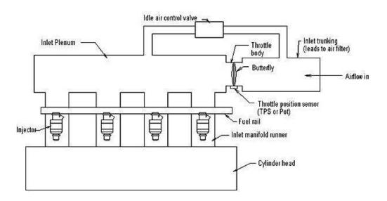
Multi point fuel injection or MPFI uses several injectors, normally respective to the number of engine cylinders and placed in the inlet port of each cylinder. It is to be noted that fuel spaying is taking place out side of the cylinder at the correct time according to the piston position inside the cylinder.
