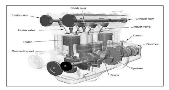
The **inline-four engine** or **straight-four engine** is a type of internal combustion four cylinder engines with all four cylinders mounted in a straight line, or plane along the crankcase. The single bank of cylinders may be oriented in either a vertical or an inclined plane with all the pistons driving a common crankshaft
