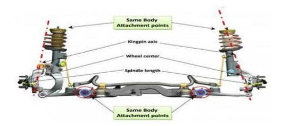
With the solid axle setup, the steering knuckle and wheel spindle assemblies are Connected to the axle beam by bronze-bushed kingpins, or spindle bolts, which provide pivot points for each front wheel. Modern independent front wheel suspension systems use ball joints, or spherical joints, accomplish the purpose. In operation, the swiveling action of the ball joints allows the wheel and spindle assemblies to be turned left and right and to move up & down with changed in roadservice.
