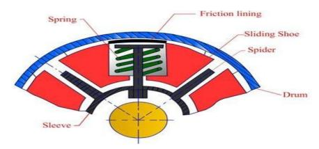
The most common types have friction pads or shoes radially mounted that engage the inside of the rim of housing. On the center shaft there are an assorted number of extension springs, which connect to a clutch shoe. When the central shaft spins fast enough, the springs extend causing the clutch shoes to engage the friction face. It can be compared to a drum brake in reverse.
