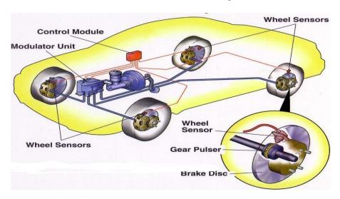
ABS generally offers improved vehicle control and decreases stopping distances on dry and slippery surfaces; however, on loose gravel or snow-covered surfaces, ABS can significantly increase braking distance, although still improving vehicle control.
