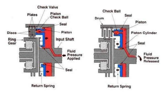
The plates are alternately fitted to the engine shaft and gear box shaft. They are firmly pressed by strong coil springs and assembled. Each of the alternate plate slides in grooves on the
