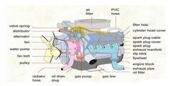
The engine is the power plant of the vehicle. In general, internal combustion engine with petrol or diesel fuel is used to run a vehicle. An engine may be either a two-stroke engine or a four-stroke engine.
