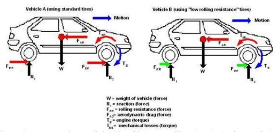
Rolling resistance, sometimes called rolling friction or rolling drag, is the force resisting the motion when a body rolls on a surface. It is mainly caused by non-elastic effects; that is, not all the energy needed for deformation of the wheel, roadbed, etc. ...
