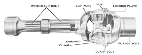
A slip joint is provided between universal joint and propeller shaft to adjust for any change in length. Slip joint allows for the change in length of propeller shaft. When spring is compressed propeller shaft shortens and when spring is expanded, propeller shaft returns to original length.
