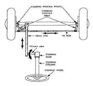
This system provides the directional change in the movement of an Automobile and maintain in a position as per the driver's decision without much strain on him.
