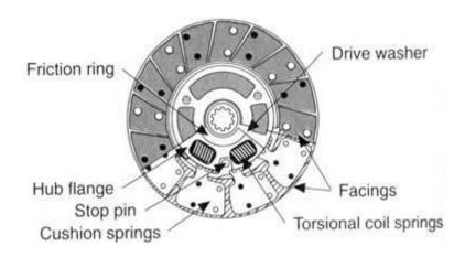
Clutch disc facing springs, also called the cushioning springs, are flat metal springs located under the friction lining of the disc. These springs have a slight wave or curve, allowing the lining to flex inward slightly during initial engagement. This also allows for smooth engagement.
