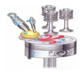
The earliest mass production multi-valve engines were 3-valves because of its simple construction - it needs only a single Camshaft to drive both intake valves and the exhaust valve of each cylinder. Today, there are still a few car cars using this cheap but inefficient design, such as Fiat Palio and all Mercedes V6 and V8 engines. Mercedes uses that because of emission rather than cost reason.
