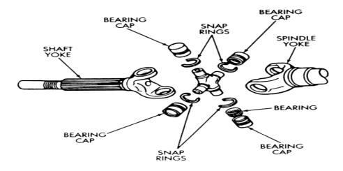
This is a variable velocity joint, i.e. the driving and driven shaft do not rotate at the same speed throughout a revolution. However, their rpm is same. This happens because both shafts are not in straight line. Ring and trunion type and cross ball type designs also come in this category of universal joints.
