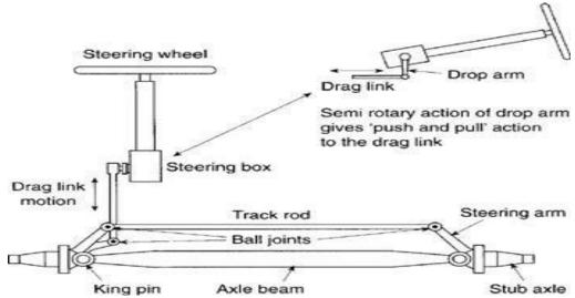
Front axles are mounted at the end of front axle. A part of the weight of vehicle is transmitted to the wheels through this axle. The front axle performs several functions.
