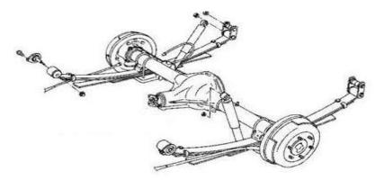
Each part of rear axle is called the half shaft. Outer end of the rear axle carries the wheel while inner end is connected to sun gear of the differential. In vehicles which employ rear wheel drive, rear wheels are driving wheels. However, in front wheel drive vehicles, front wheels are driving wheels. Rear axles and differential are completely enclosed in a housing to protect them from dust, dirt, water and any possible damage.
