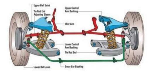
Suspension system of an automobile separates the wheel and axle assembly of the automobile from its body. Main function of the suspension system is to isolate the body of the vehicle from shocks and vibrations generated due to irregularities on the surface of roads. Shock absorbers are provided in the vehicles for this purpose. It is in the form of spring and damper. The suspension system is provided both on front end and rear end of the vehicle.
