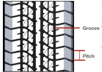
**Groove:-** The groove is the hollow part or the tread. The grooves are cut which makes the tyre pattern. Tyres come in different patterns and grooves, from the simple block pattern to the modern v tread designs. The hollow part (the groove) is designed to channel the water out and away. As a the tread wears the groove becomes less hollow and apparent. The design of the groove effects the performance and the quality of the tyre.
