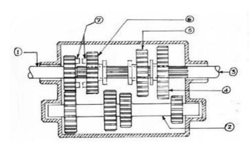
1.Main drive gear 2.Counter shaft 3.Main shaft 4.I gear 5.II gear 6.III gear 7.Top speed engaging dogs
