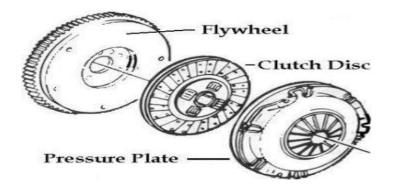
The purpose of the clutch is to disconnect the engine from the driven wheels when a vehicle is changing gears or being started from rest.
