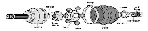
This type of joint permits movement of both driving and driven shafts at constant velocity. Because, two joints in this case operate at same angles. These joints are generally used when the automobile in a front wheel (axle) drive. Because speed variation between driving and driven shaft will introduce difficulty in steering and excessive tyre wear.
