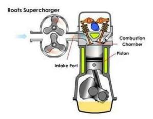
Both turbochargers and superchargers are called **forced induction systems**. They compress the air flowing into the engine .The advantage of compressing the air is that it lets the engine stuff more air into a cylinder. More air means that more fuel can be stuffed in, too, so you get more power from each explosion in each cylinder. A turbo/supercharged engine produces more power overall than the same engine without the charging.
