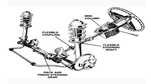
In front wheels can be turned to left and right by steering system so that the vehicle can be steered. The steering wheel is placed in front of driver. It is mechanically linked to the wheels to provide the steering control. The primary function of the steering system is to provide angular motion to front wheels so that vehicle can negotiate a turn. It also provides directional stability to vehicle when the vehicle moves ahead in straight line.
