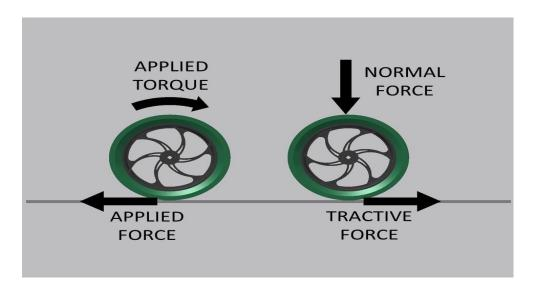
As used in automobile engineering, the term tractive force can either refer to the total traction a vehicle exerts on a surface, or the amount of the total traction that is parallel to the direction of motion.
