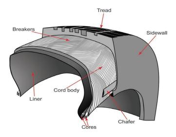
This provides a strong, stable casing, with relatively stiff side walls. However during cornering, stiff sidewalls can distort the tread and partially lifting it off the road surface. This reduces the friction between the road and the tyre. Stiff sidewalls can also make tyres run at a high temperature. This is because, as the tyre rotates, the cords in the plies flex over each other, causing friction and heat. A tyre that overheats can wear prematurely.
