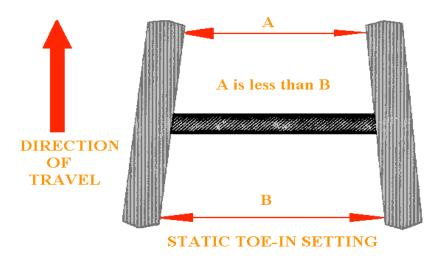
It is the amount in minimum at the front part of the wheel points inwards approximately 3 to 5 mm. It prevents side slipping excessive tyre wear, proper rolling of front wheels and steering stability.
