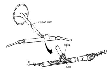
This is common manual type of steering gear box is used in most of the vehicles. In this type of steering a pinion is provided the bottom end of the steering column. The teeth of the pinion wheel in mesh with corresponding teeth provided on the rack, the end of which is connected to the stub axle through the rod. The rotating motion of the pinion operates the rack in FORE and AFT direction which in turn operates the stub axle.
