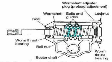
The balls are recirculated through the ball guides.
