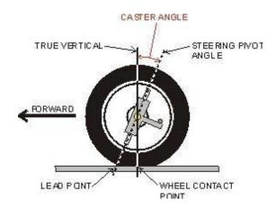
This is the angle between backward or forward tilting of the king pin from the vertical axis at the top. This is about 2° to 4°. The backward Tilt is called as positive caster. The forward tilt is called negative caster.
