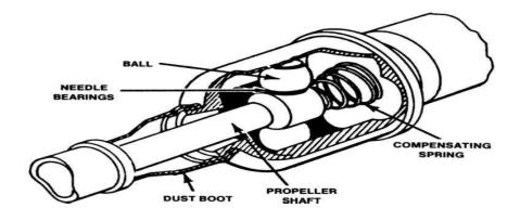
This type of joint consists of a ball type head which is fastened to one end of the propeller shaft. A pin is also pressed through this end of shaft. Two steel balls are fitted at the end of this pin. The joint facilitates rotary motion through ball and pin. The balls can also move axially. Ball and trunnion joint is also a variable velocity joint.
