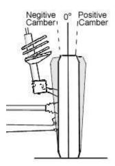
The angle between wheel axis to the vertical line at the top is called camber angle. It is approximately  $\frac{1}{2}$ ° to 2°.
