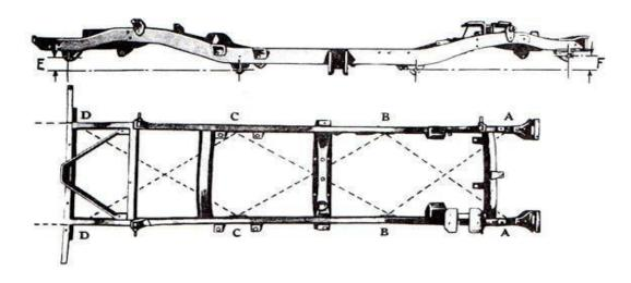
The frame is the main part of the chassis on which remaining parts of chassis are mounted. The frame should be extremely rigid and strong so that it can withstand shocks, twists, stresses and vibrations to which it is subjected while vehicle is moving on road. It is also called underbody.
