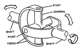
A universal joint takes care of rising and falling motion of the rear end of the propeller shaft which is connected to differential.
