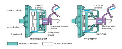
When the operator releases the clutch pedal, spring pressure inside the pressure plate pushes forward on the clutch disc. This action locks the flywheel, the clutch disc, the pressure plate, and the transmission input shaft together. The engine again rotates the transmission input shaft, the transmission gears, the drive train, and the wheels of the vehicle.
