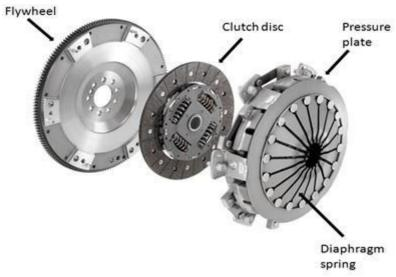
The flywheel is the mounting surface for the clutch. The pressure plate bolts to the flywheel face. The clutch disc is clamped and held against the flywheel by the spring action of the pressure plate. The face of the flywheel is precision machined to a smooth surface. The face of the flywheel that touches the clutch disc is made of iron. Even if the flywheel were aluminum, the face is iron because it wears well and dissipates heat better.
