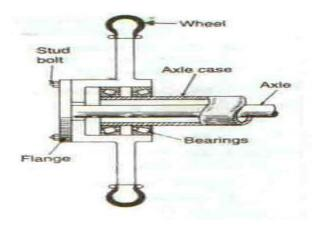
In fully floating rear axle, the bearings are provided between axle casing and the wheel. In this case, all the vehicle weight is transmitted to ground through axle case and wheel. The axle is not supported by bearings but it is supported at both ends. This type of axle is very strong and therefore, it is used for heavy duty vehicles. In the event of breakdown of axle, wheel cannot come out. This, it is safer but costly.
