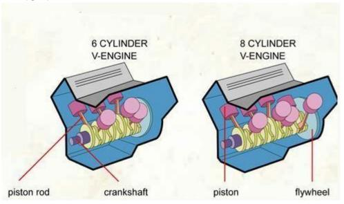
**Vee engine** is a common configuration for an internal combustion engine. The cylinders and pistons are aligned, in two separate planes or 'banks', so that they appear to be in a "V" when viewed along the axis of the crankshaft. The Vee configuration generally reduces the overall engine length, height and weight compared to an equivalent inline configuration.
