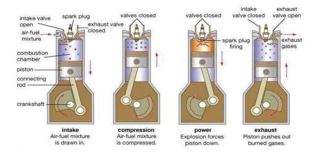
A **four-stroke engine** (also known as **four-cycle**) is an internal combustion engine in which the piston completes four separate strokes which comprise a single thermodynamic cycle. A stroke refers to the full travel of the piston along the cylinder, in either direction. While risqué slang among some automotive enthusiasts names these respectively the "suck," "squeeze," "bang" and "blow" strokes. They are more commonly termed
