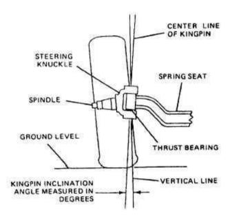
It is the angle between vertical line to the king pin axis. The inclination tends to keep wheels straight ahead and make the wheels to get return to the straight position after completion of a turn. The inclination is normally kept 7° to 8°
