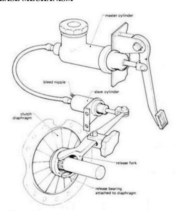
A hydraulic clutch release mechanism uses a simple hydraulic circuit to transfer clutch pedal action to the clutch fork. It has three basic parts—master cylinder, hydraulic lines, and a slave cylinder. Movement of the clutch pedal creates hydraulic pressure in the master cylinder, which actuates the slave cylinder. The slave cylinder then moves the clutch fork.
