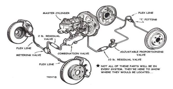
Brakes are used to slow down or stop the vehicle. Hydraulic brakes are generally used in automobiles, where brakes are applied by pressure on a fluid. Mechanical brakes are also used in
