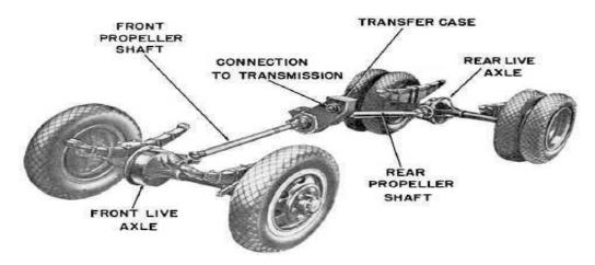
Four-wheel drive, 4WD, 4x4 ("four-by-four"), all-wheel drive, and AWD are terms used to describe a four-wheeled vehicle with a drivetrain that allows all four roadwheels to receive torque from the internal combustion engine simultaneously. This system is common in off-road vehicles - powering all four wheels provides better control on loose and slippery surfaces. It is often used in rally racing on mostly-paved roads.
