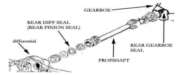
Final drive is the last stage in transferring power from engine to wheels. It reduces the speed of the propeller shaft (drive shaft) to that of wheels. It also turns the drive of the propeller shaft by an angle of 900 to drive the wheels.
