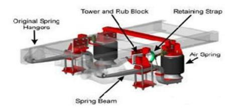
A typical air suspension system consists of an engine-driven air compressor, supply tank, filter or condenser, valves, piping, controls and air springs or bellows in operation, the air compressor maintains a constant pressure in the supply tank. Air is piped to the control valves, which feed air to each spring as needed. Pressure is automatically increased on either side or at front or rear as required to keep the car level and to keep any desired height from the road (within limit of system).
