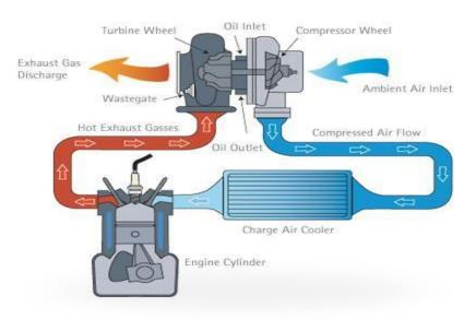
The key difference between a turbocharger and a supercharger is its **power supply**. Something has to supply the power to run the air compressor. In a supercharger, there is a **belt** that connects directly to the engine. It gets its power the same way that the water pump or alternator does. A turbocharger, on the other hand, gets its power from the **exhaust stream**. The exhaust runs through a turbine, which in turn spins the compressor.
