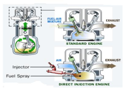
Direct fuel injection is a fuel-delivery technology that allows gasoline engines to burn fuel more efficiently, resulting in more power, cleaner emissions, and increased fuel economy.
