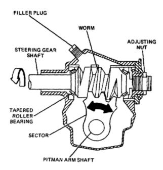
In this type the worm on the end of the steering shaft meshes with a sector mounted on a sector shaft. When the worm is rotated by rotation of the steering wheel, the sector also turns rotating the sector shaft. Its motion is transmitted to the wheel through the linkage. The sector shaft is attached to the drop arm or pitmen arm.
