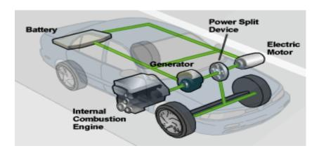
A hybrid vehicle is a vehicle that has two sources of power. A typical hybrid vehicle will have a fuel-driven combustion engine along with a rechargeable system for storing energy. A hybrid vehicle may also have other power sources such as a mechanism to utilize the power of the wind. Alternatively, the vehicle may use mechanical power like the pedaling motion of an individual. Based on the engine used, a hybrid vehicle may be classified into parallel and series type.
