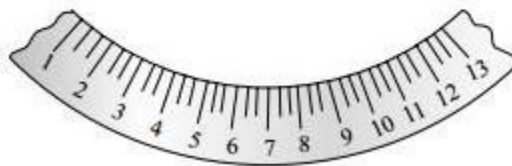
(b) Vertical circle graduations (20' main scale)
