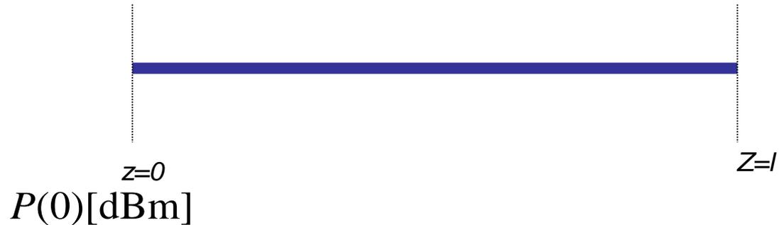
$$P(l)[\text{dBm}] = P(0)[\text{dBm}] - \alpha[\text{dB/km}] \times l[\text{km}] \quad [3-3]$$
