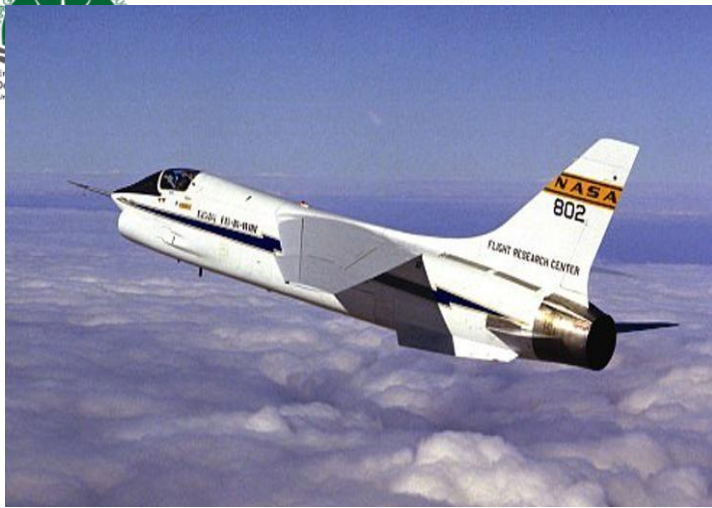
F-8C Crusader Digital fly-by-wire test bed (1972)
