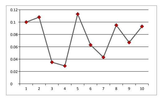
Since all the sample points lie with in the control lines, the process is under control.
