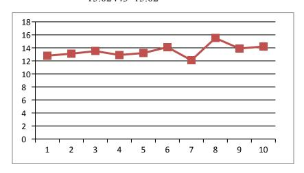
Conclusion: Since 8th sample mean fall outside the control limits the statistical process is out of control according to chart
