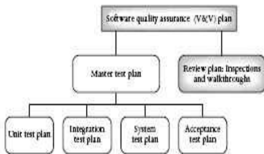
FIG. 7.1 A hierarchy of test plans.
