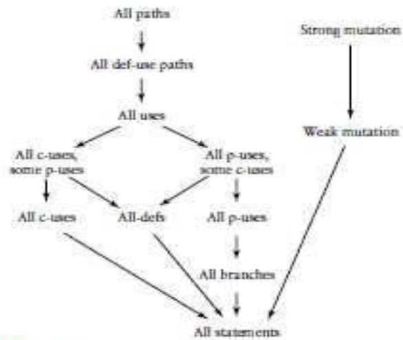
FIG. 5.5 A partial ordering for test adequacy criteria.
