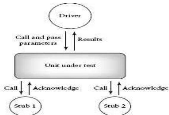
Fig. 6.5 The test harness.
