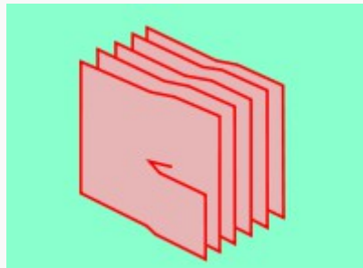
Figure C Schematic diagram (lattice planes) showing a screw dislocation.
