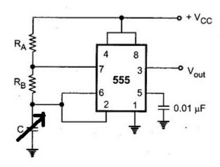
$RA=10K\Omega$ ,  $RB=100K\Omega$ ,  $C1=0.01\mu f$
