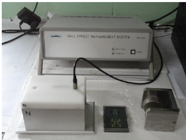
Hall effect measurement system used for present work
