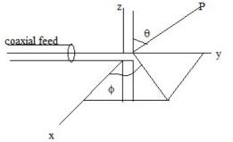
The resistance Rr is called radiation resistance. It is the resistance which would dissipate the same power than the current element. A simple example of current element radiator is a centre fed short linear antenna whose length dl is small compared to wavelength  $\lambda$ .
