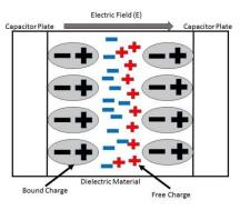
Using the capacitor model, it is possible to define the relative permittivity or the dielectric constant of the material by setting its relative permittivity equivalent to the ratio of the measured capacitance and the capacitance of a test capacitor, which is also equal to the absolute permittivity of the material divided by the permittivity of a vacuum.
