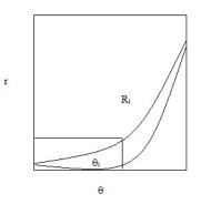
Further fro the curves it is clear that the reflecting power at normal incidence is 4% only and it falls to zero at polarising angle for the light with vibration in the plane of incidence and for light with its vibration Ito the plane of incidence it is 15%. All the light is reflected as the angle of incidence approaches  $90^{\circ}i.e$  grazing angle.
