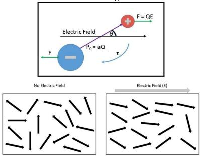
To determine if the induced average dipole moment along the electric field, the average potential energy of the dipole must be calculated and compared to the average thermal energy 1/5kT, as determined by thermodynamics for five degrees of freedom. To accomplish this, Force F torque  $\tau$  acting on the rigid body of the dipolar molecule. Using this model, the equation for the torque is given by
