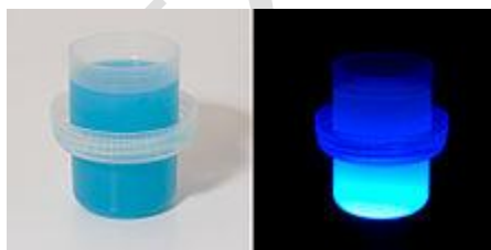
Laundry detergent fluorescing under ultraviolet light
