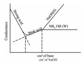
Conductometric titration of a mixture of a strong acid (HCl) and a weak acid (CH<sub>3</sub>COOH) vs. a strong base (NaOH) or a weak base (NH<sub>4</sub>OH)
