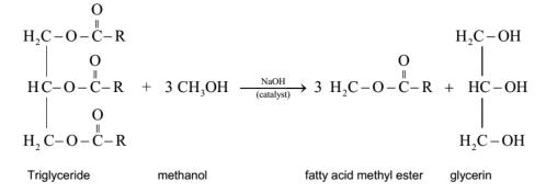
The preparation of the biodiesel is a transesterification reaction where the triglycerides are converted into simpler methyl esters of the fatty acids (the biodiesel).
