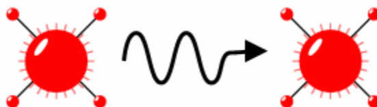
Fig3: Recoil-free emission or absorption of a gamma-ray when the nuclei are in a solid matrix such as a crystal lattice
