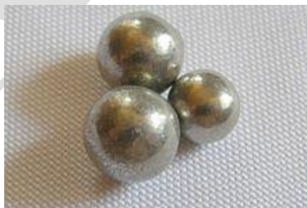
Spheres of nickel manufactured by the Mond process
