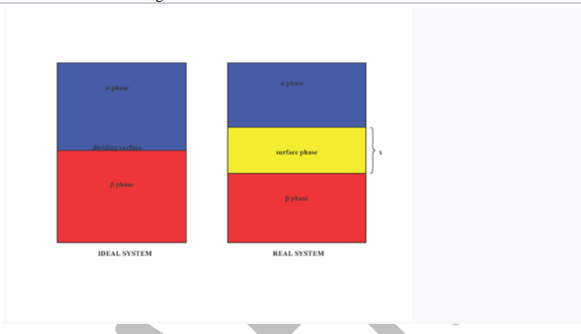
Figure : Comparison between the real and idealized models of the surface
