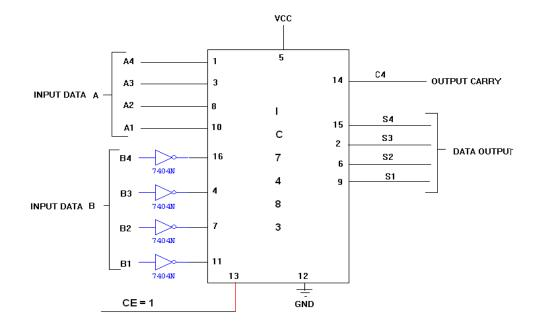
LOGIC DIAGRAM: 4-BIT BINARY ADDER/SUBTRACTOR
