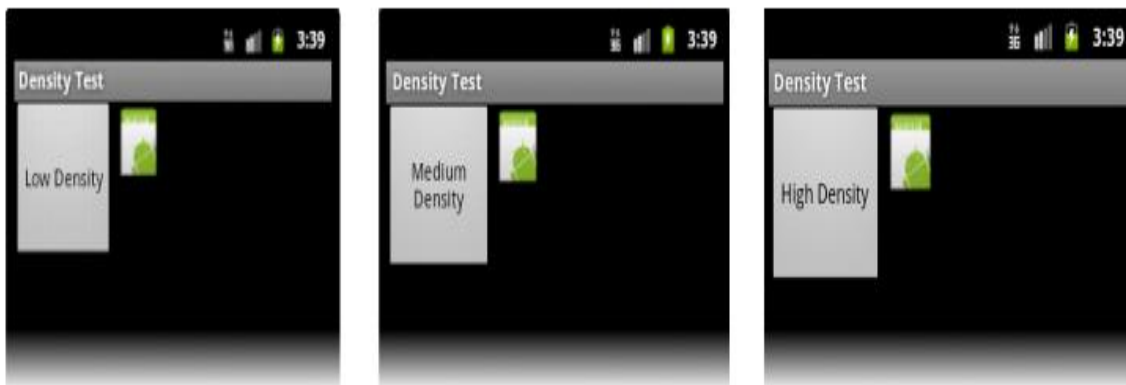
Figure 3. Example application with good support for different densities (it's density independent), as shown on low, medium, and high density screens.
