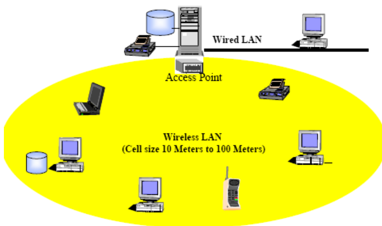
Figure4-1: A Simple Wireless LAN Configuration
