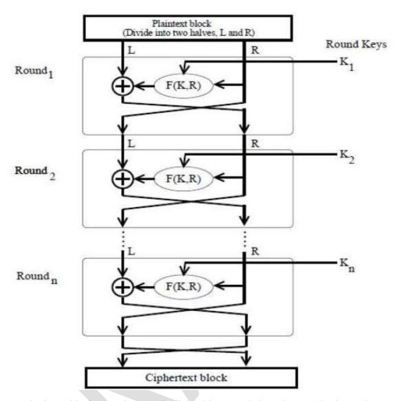
The input block to each round is divided into two halves that can be denoted as L and R for the left half and the right half.
