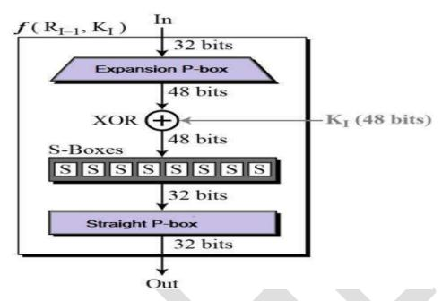
**Expansion Permutation Box** – Since right input is 32-bit and round key is a 48-bit, we first need to expand right input to 48 bits. Permutation logic is graphically depicted in the following illustration –
