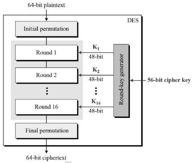
Since DES is based on the Feistel Cipher, all that is required to specify DES is –
