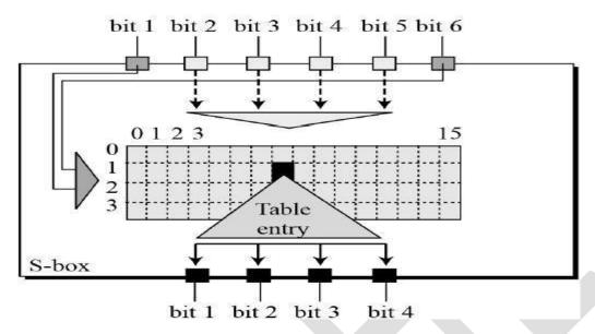
There are a total of eight S-box tables. The output of all eight s-boxes is then combined in to 32 bit section.
