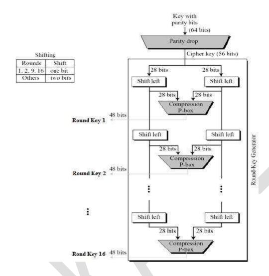
The logic for Parity drop, shifting, and Compression P-box is given in the DES description
