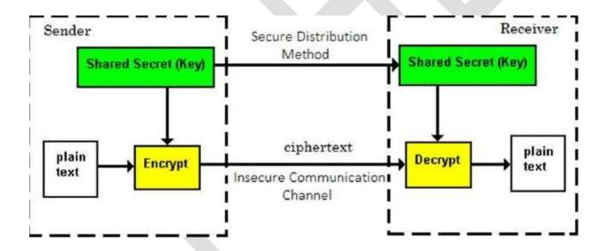
all cryptosystems employed symmetric key encryption. Even today, its relevance is very high and it is being used extensively in many cryptosystems. It is very unlikely that this encryption will fade away, as it has certain advantages over asymmetric key encryption.
