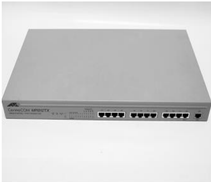
FIGURE 3.2 A high-capacity, or high-density, hub.
