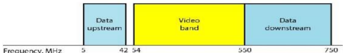
Figure 1.61 Division of coaxial cable band by CATV
