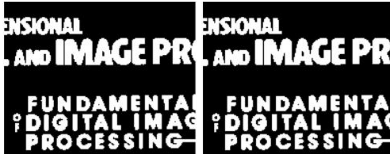
Opening: a 2×2 square structuring element
