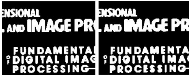
Closing: a 2x2 square structuring element
