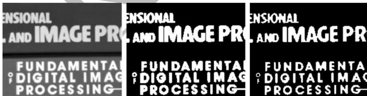
Erosion: a 2×2 square structuring element
