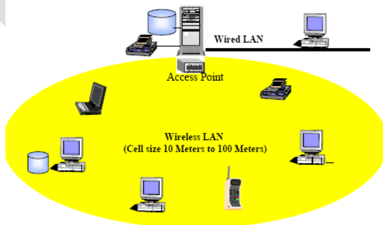
Figure4-1: A Simple Wireless LAN Configuration
