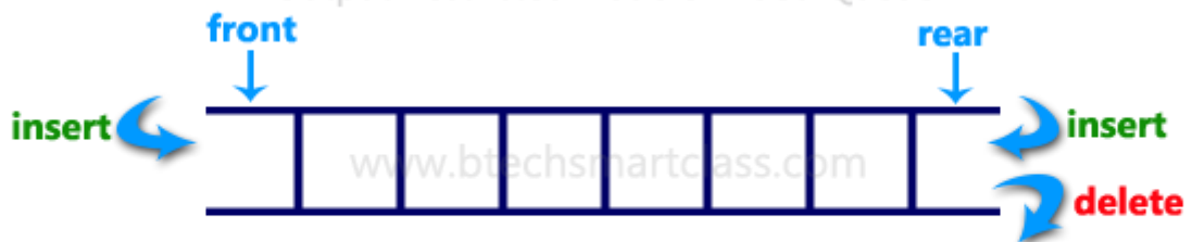
Output Restricted Double Ended Queue
