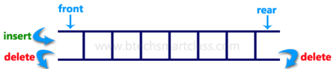
Input Restricted Double Ended Queue
