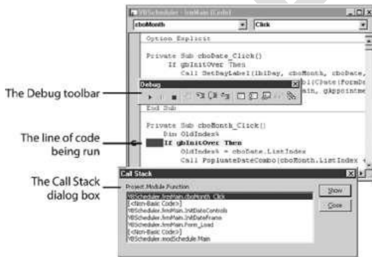
Figure 7.9 Debugger allows to single-step through the software to see lines of code and modules are executed while running test cases.
