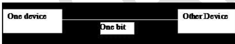
Figure 5.2: Serial transmission - one bit at a time
