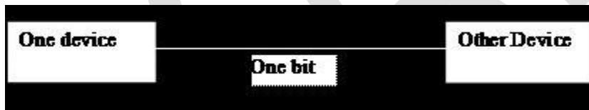
Figure 5.2: Serial transmission - one bit at a time
