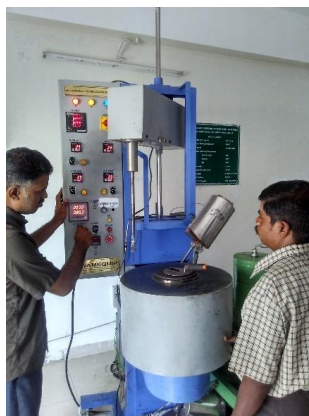
22.04.2017 - Manufacturing of Composite in Stir Casting Machine
